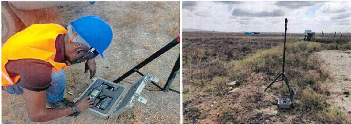
Noise monitoring garget set up within wildlife conservancy area in specific geological coordinates to know effects of noise and vibration to nesting birds.
